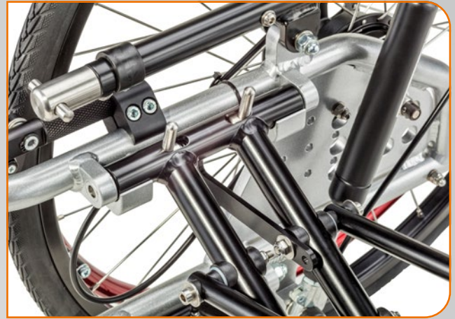
Entriegelung Faltmechanik unlocking folding mechanism
