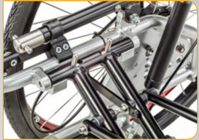
Entriegelung Faltmechanik unlocking folding mechanism
