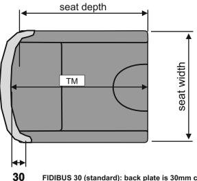
FIDIBUS 30 (standard): back plate is 30mm curved FIDIBUS 50 : back plate is 50mm curved
