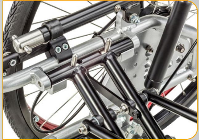
Entriegelung Faltmechanik unlocking folding mechanism
