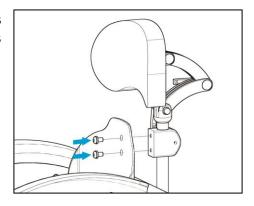
To adjust the headrest to the person, you must loosen the respective clamping levers, then you can adjust the height and position of the headrest according to your requirements.
