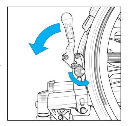
After adjustment, please make sure that you have tightened all screw connections again so that the brake cannot come loose.
