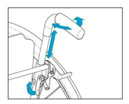
The described possibility of removing the push handles without tools has the advantage of being able to remove them at any time, e.g. for transporting/loading the wheelchair. However, the disadvantage is that the wheelchair no longer offers adequate grip options for pushing the wheelchair when the push handles have been removed!
