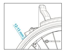
To adjust the brake, i.e. to change the distance between the tyre and the pressure lever, you must first loosen the nut on the inside of the brake mechanism.
