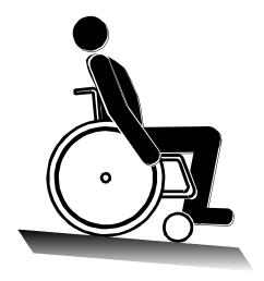
Notice that the footrests do not contact the ground at the end of a slope as a suddenly, unwanted braking could danger you.
