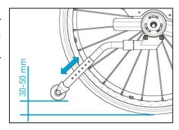
The device is screwed onto the axle mount from below with two screws.
