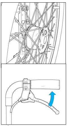
**Note:** Uneven actuation of the two brake levers produces cornering.
